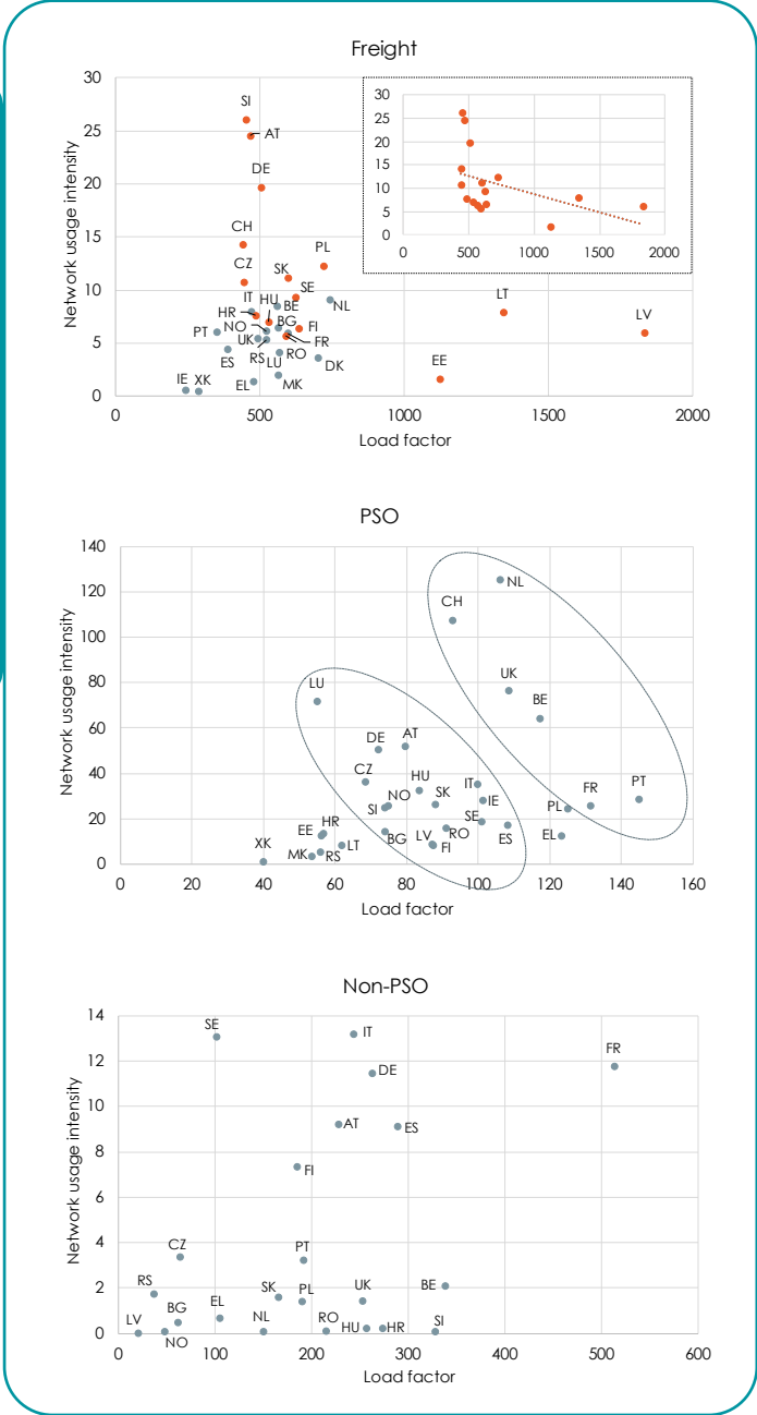
Figure 34 – Relationship between network usage intensity (train-km per route km per day) and train load factor (passenger-km or tonne-km per train-km) per country in 2022 36
